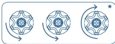
The angle of the shift must be greater than 2 degrees as compared to the rest position.
